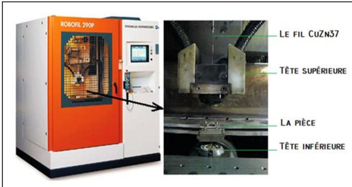
**Figure 14.** La machine ROBOFIL 290P.
