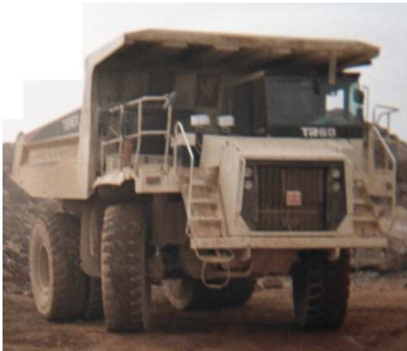
Figure IV.3 : Dumper TEREX TR60.
