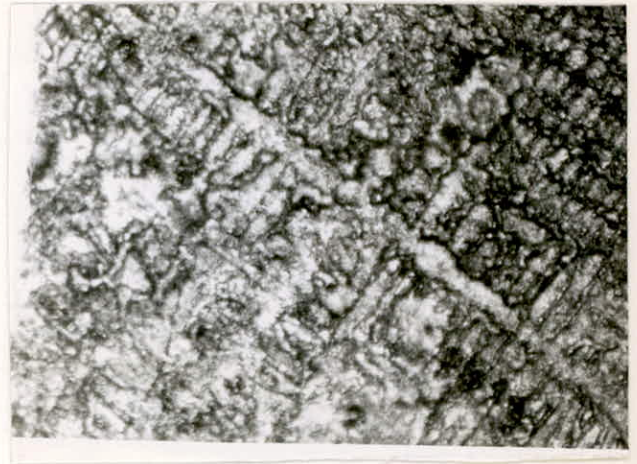
Pb - Cu (0,043%) - Sb (0,77%) X 125 large grain dendritique de Pb (Blanc)
