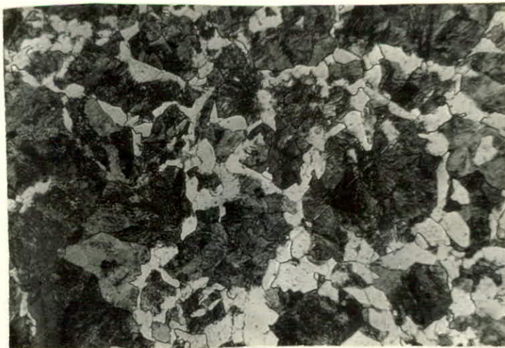
Attaque au Nital 5%. x 350 Zone de Transition: 50% Pearlite, 50% Ferrite.
