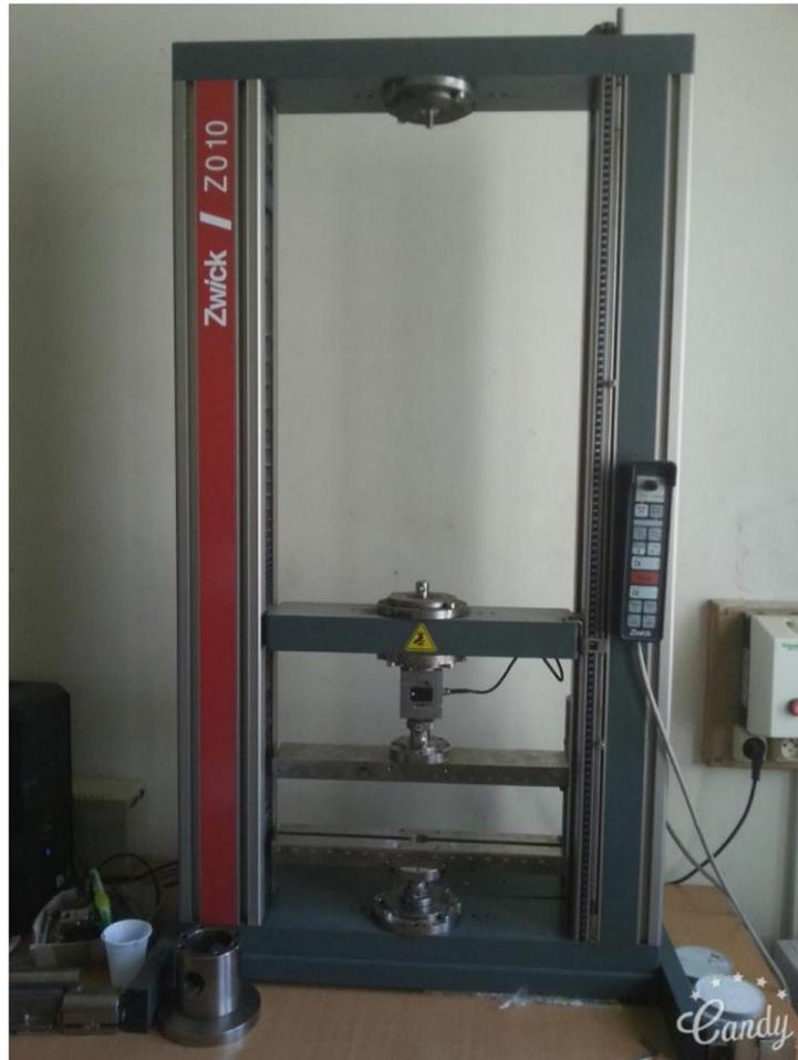
Figure II.3. Machine de compression Zwick/Roell
