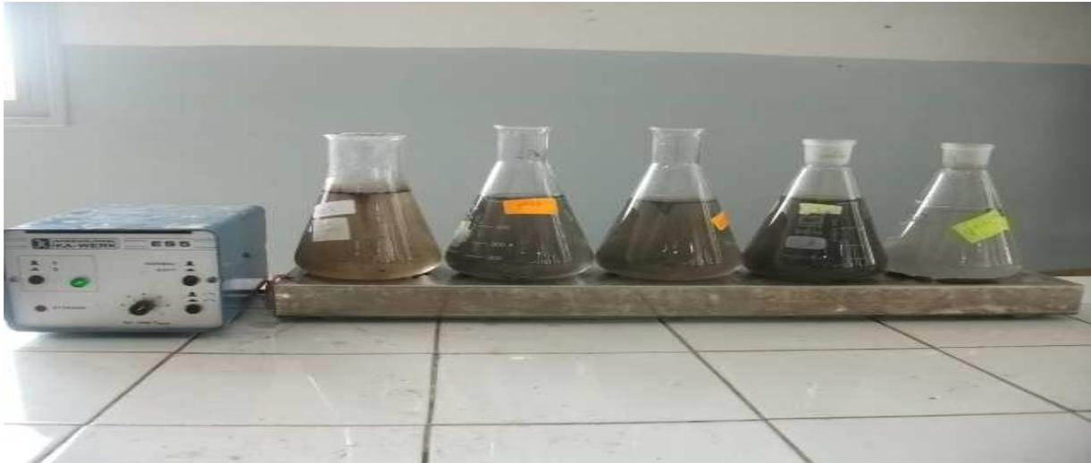
**Figure V.18:** Adsorption en batch
