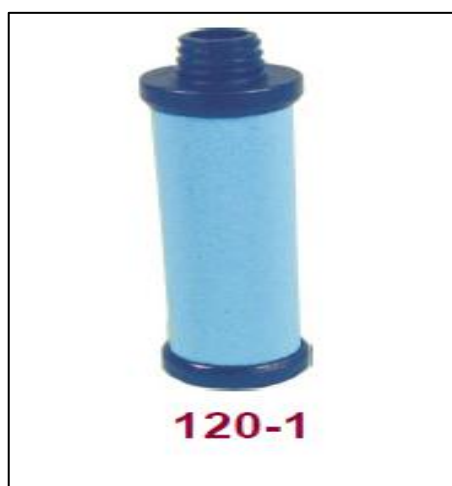
Figure n°18: Corps diffusif Radiello code 120-1
