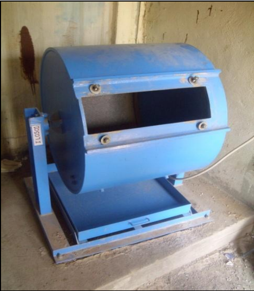
Figure IV.5. Machine Los Angeles
