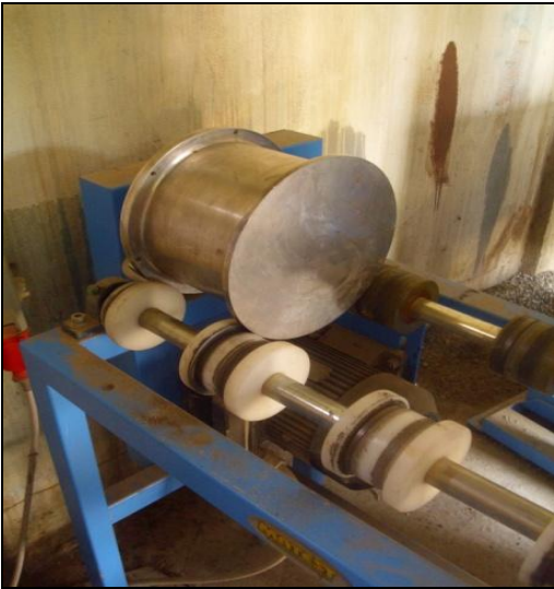
Figure IV.4. Machine Micro Deval
