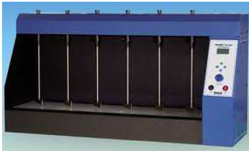
Figure III.1 : Flocculateur (Jar test)
