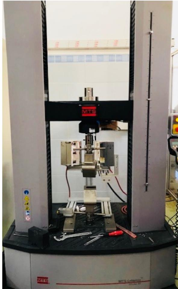
FIGURE 4.15 – La machine de traction
