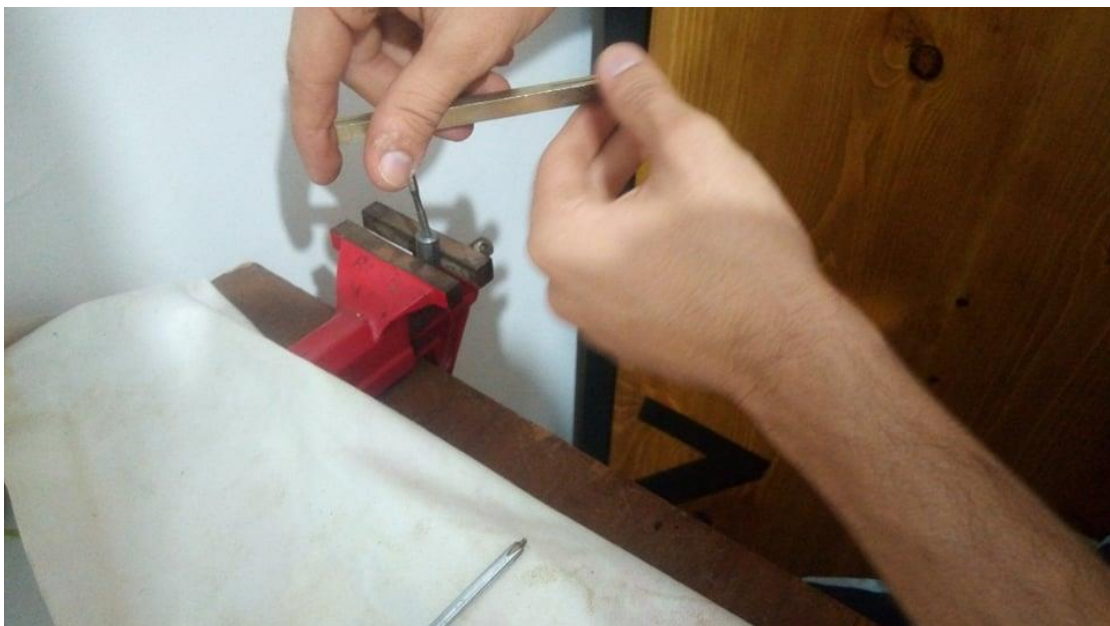
FIGURE III.19 Taraudage des pines
