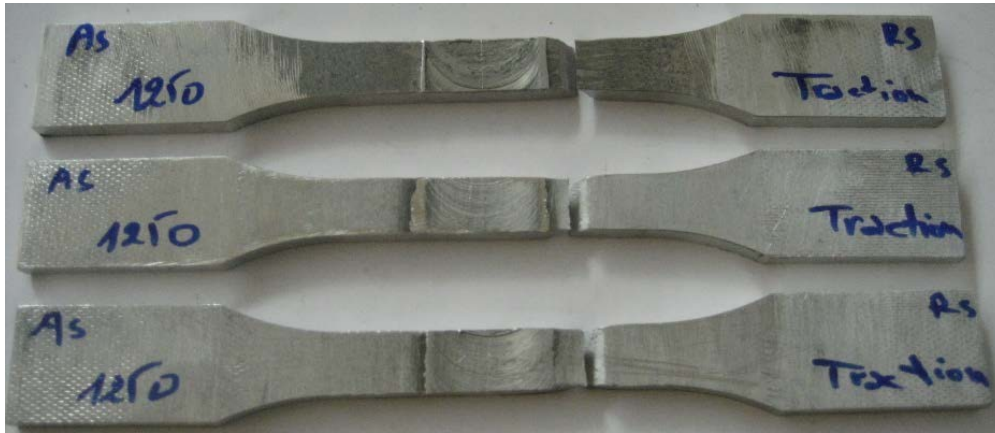
FIGURE 3.17: Rupture hors joints de soudure.
