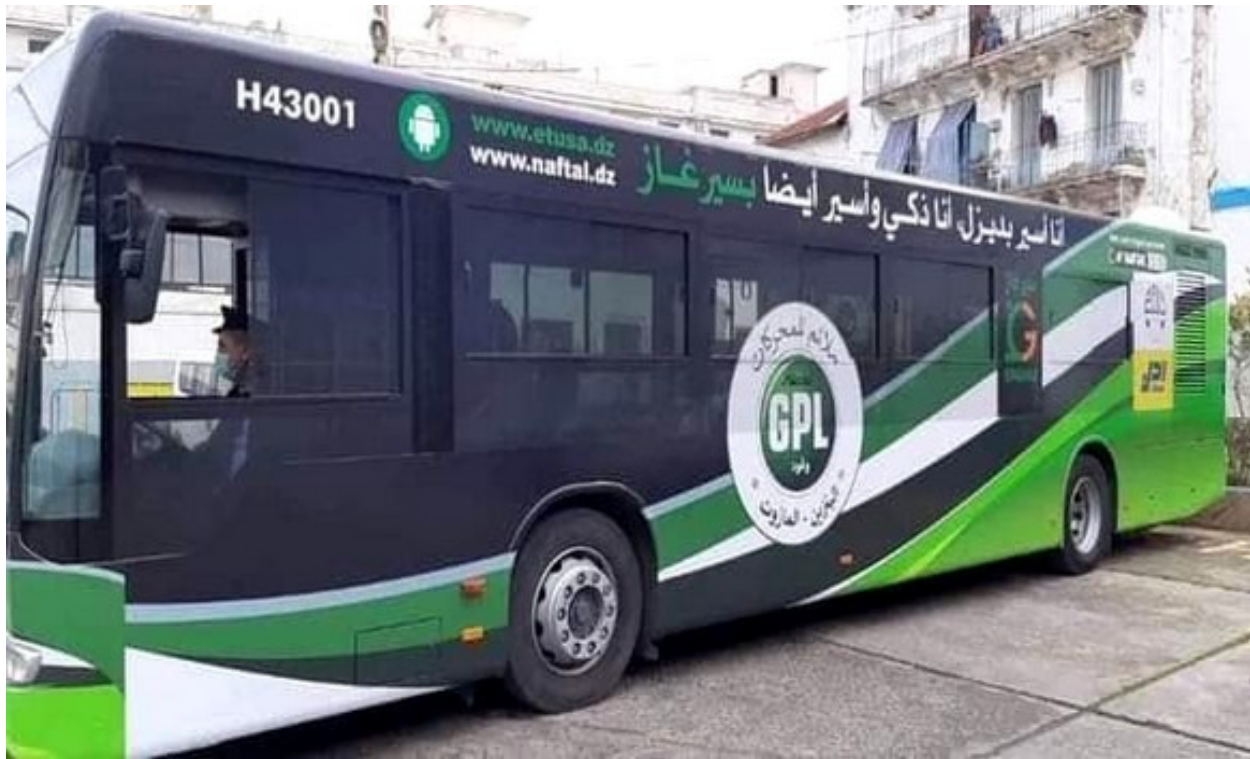
Figure 6 The first public transport bus operating in LPG-diesel dual fuel mode in Algeria [18]
