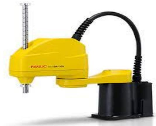
FIGURE 1.3: Robot SCARA Fanuc SR-3iA
