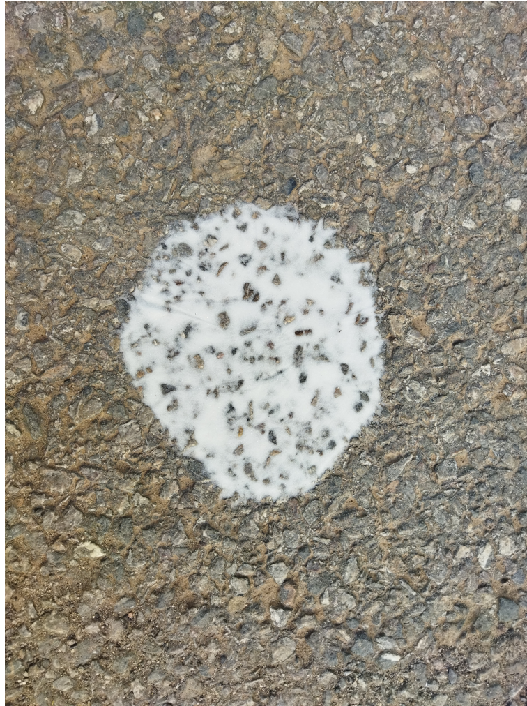
Figure 6.6: The sand patch method
