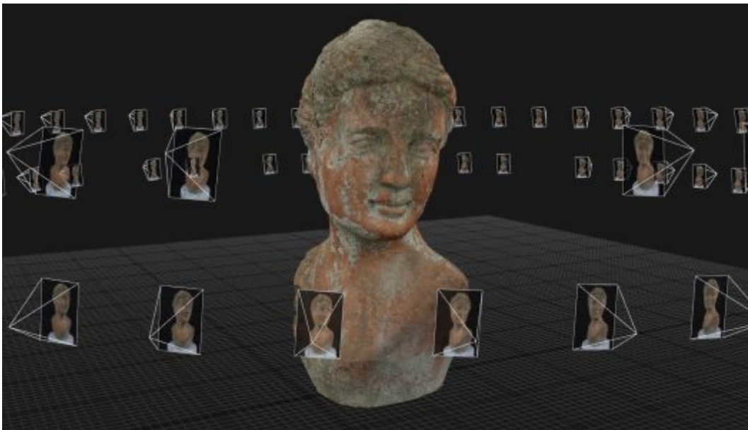
Figure 2.2: A 3D model of a statue reconstructed using photogrammetry
