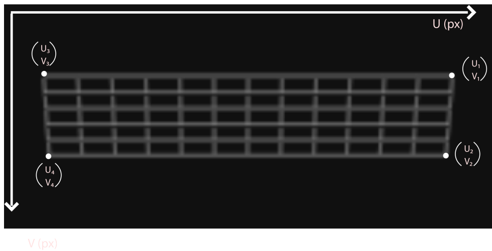
Figure 3.5: Image of the grid with the real coordinates
