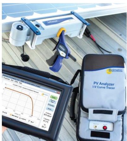
(a) IV-curve tracer for PV modules / strings / arrays, up to 1500V / 30A PV Analyzer Solmetric
