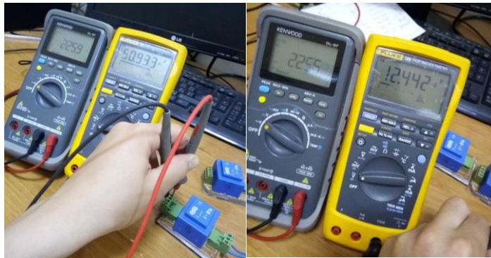
Figure 2.20 Calibration of AC voltage transformers with multimeter.
