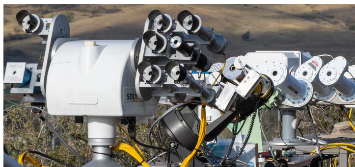
Figure 1.23 Pyrheliometer measurement comparison 2018. (Source: NREL)
