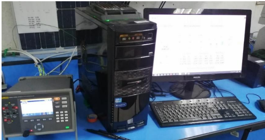
Figure 2.45 Meteorological and electrical data monitoring measured using Fluke 2638A & LabVIEW.
