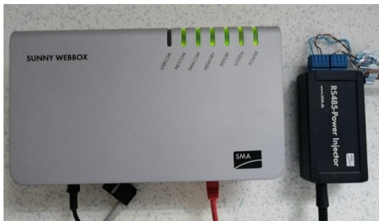
Figure 2.4 Picture of SMA SUNNY WEBBOX with RS485-Power Injector
