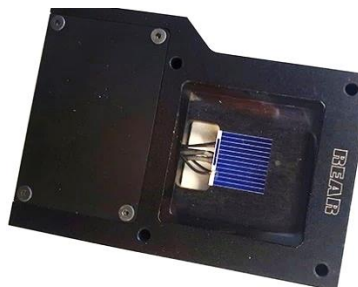
Bifacial Reference Cell (rear face) from ReRa Systems
