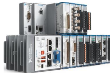
(c) Real-time DAQ (NI - CompactRIO)
