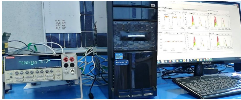
Figure 2.39 Monitoring of GCPV system using Keithley 2700 DAQ under LabVIEW.
