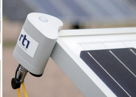
Figure 1.21 Silicon-cell Pyranometer rt1 (Class C). (source: kipp & zonen)
