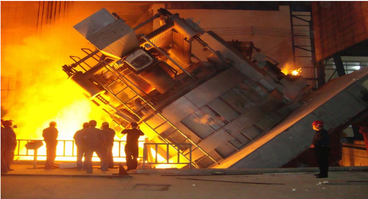
Figure II.7: L'extraction des scories.
