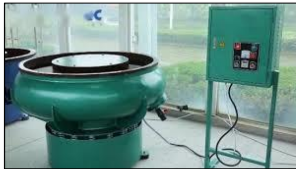
Figure 1-10 - Tonneau vibrant de tribofinition
