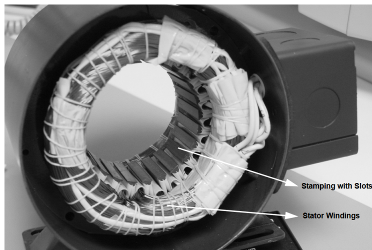
FIG. 3.11 : STATOR OF A BLDC MOTOR[21].
