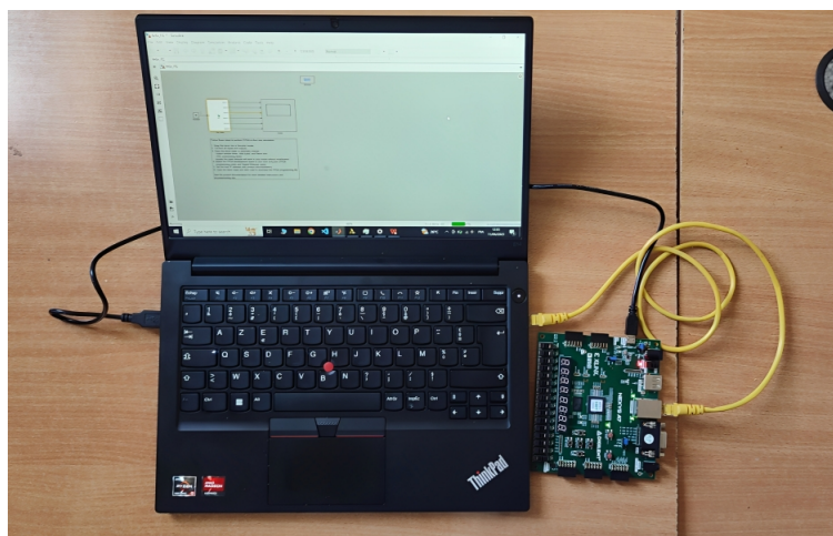
Figure 5.1: FPGA in the loop using NEXYS A7
