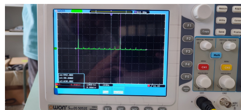
(b) FFT of the inverter's output with ASM
