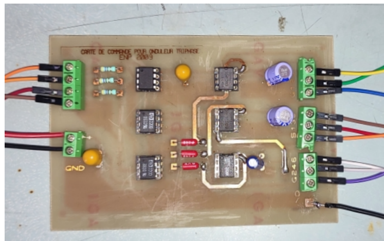
Figure 5.7: inverters command card
