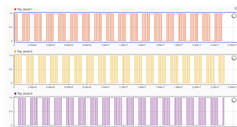
(a) Three phased ANNSHE PWM signals and the output of the FPGA
