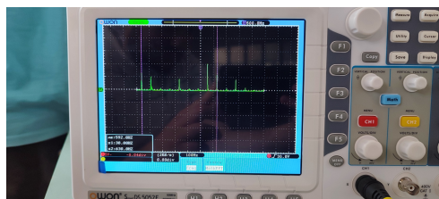
(a) FFT of the inverter's output without ASM
