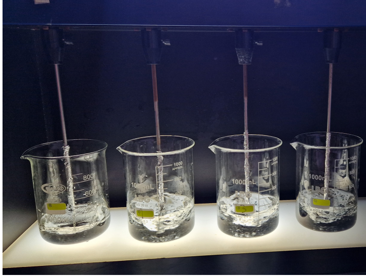
Figure 4.2: Experimental set-up of the adsorption isotherms
