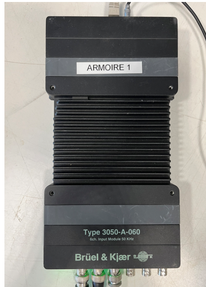
FIGURE 2.13 – Centrale d'acquisition Brüel &amp; Kjær
