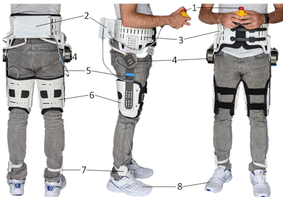
Figure 3.1 – E-Walk V1 hardware components: 1) emergency stop button, 2) embedded controller enclosure, 3) torso attachment, 4) motors, 5) thigh segments, 6) thigh attachments, 7) foot sensor amplifier boards, 8) instrumented shoes
