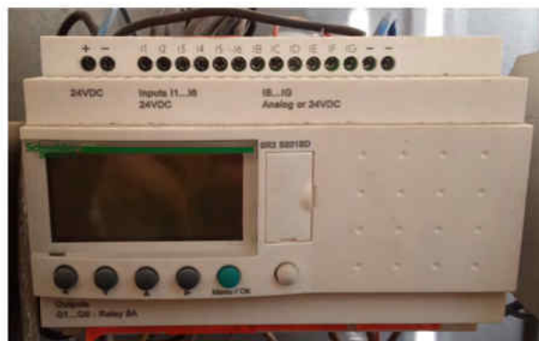
FIGURE 2.1 – Automate Zelio Logic SR2 B201BD
