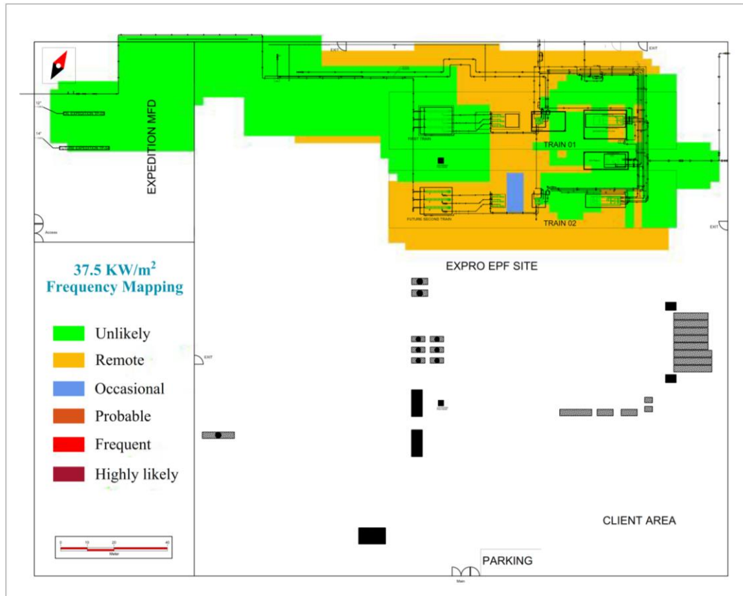
Figure 5-1 Frequency Mapping for 37.5 \text{ kW.m}^{-2} Thermal Radiation Intensity
