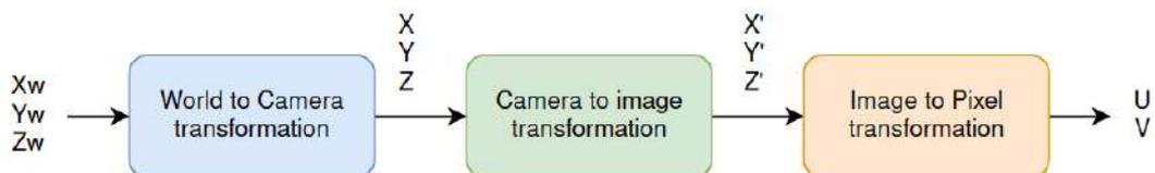
Figure 2.2: The transformation pipeline
