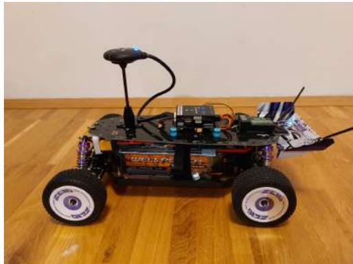
Figure 1.7: a rover controlled by PX4.
