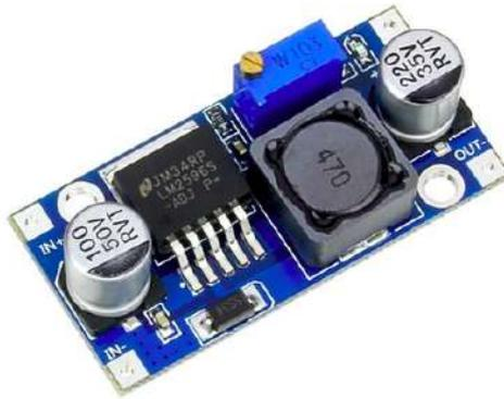
Figure 3.10: LM2596 Adjustable DC-DC Voltage regulator
