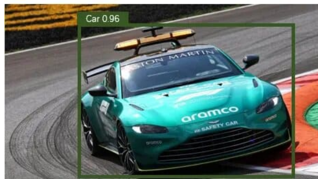
(a) the model has a 96% confidence that the object in the box is a car
