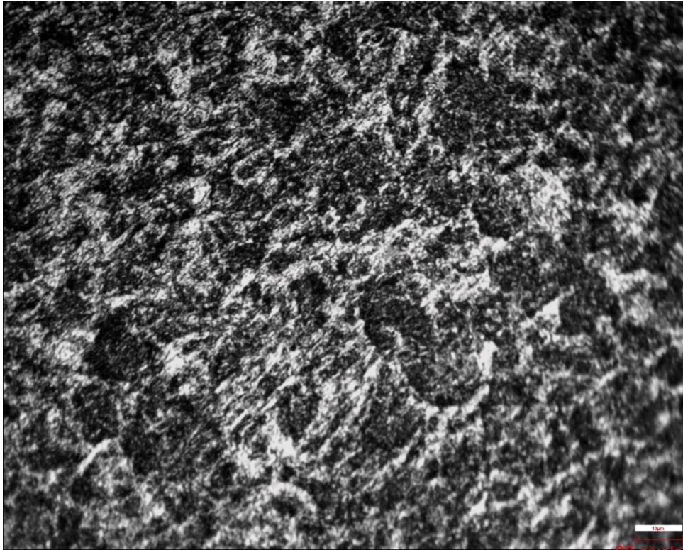
Figure 30. 280A HAZ Microstructure
