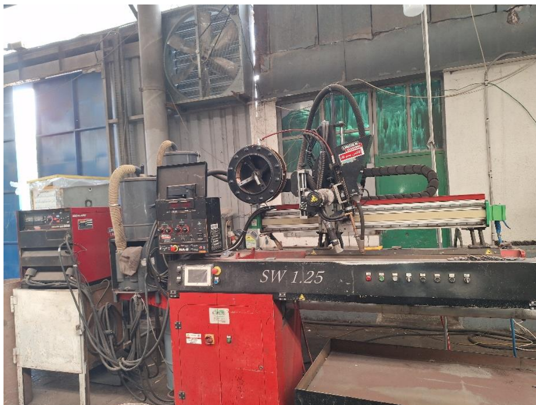
Figure 14. Welding Equipment (NUOVA CMM SW 1.25 and Lincoln Electric Idealarc® DC600)
