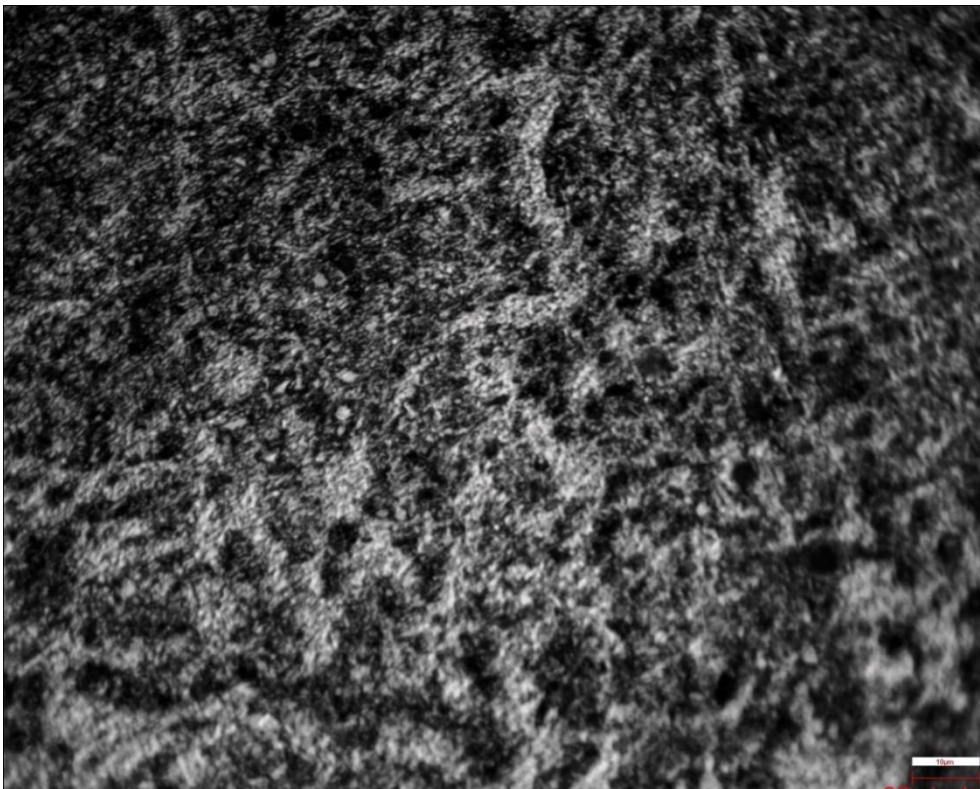
Figure 29. 280A Weld Zone Microstructure
