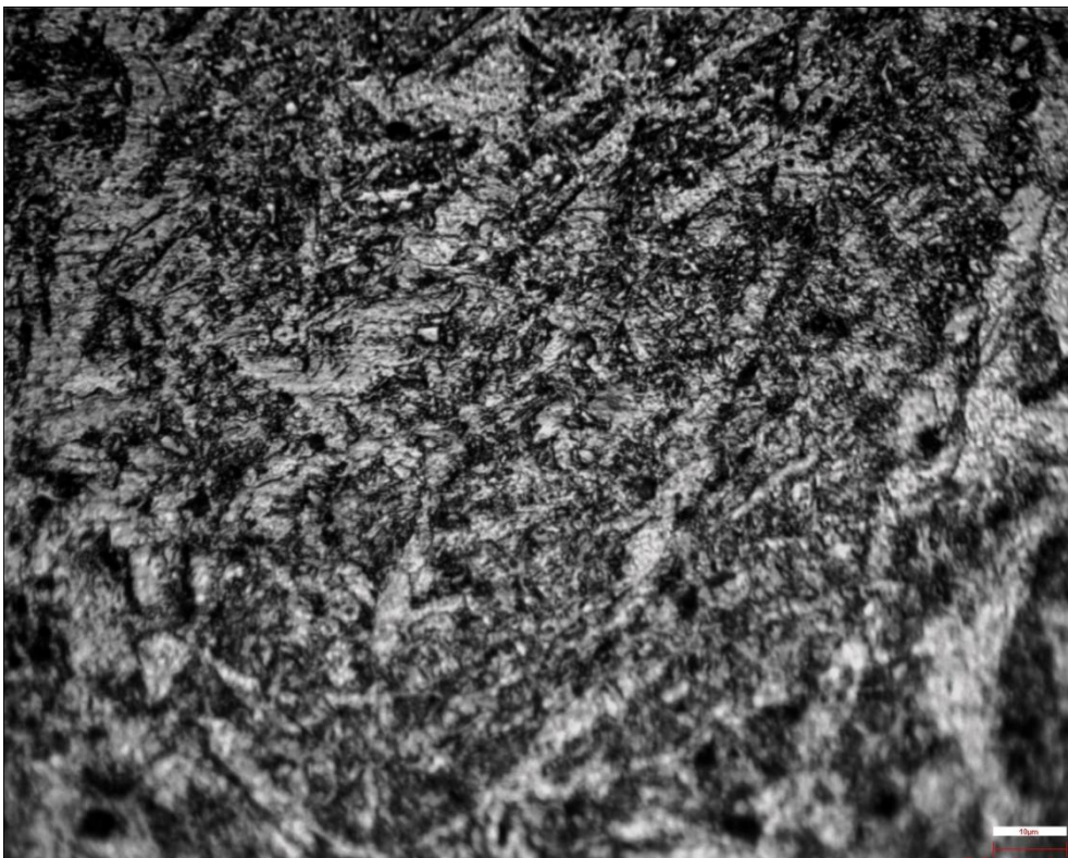
Figure 33. 350A Weld Zone Microstructure
