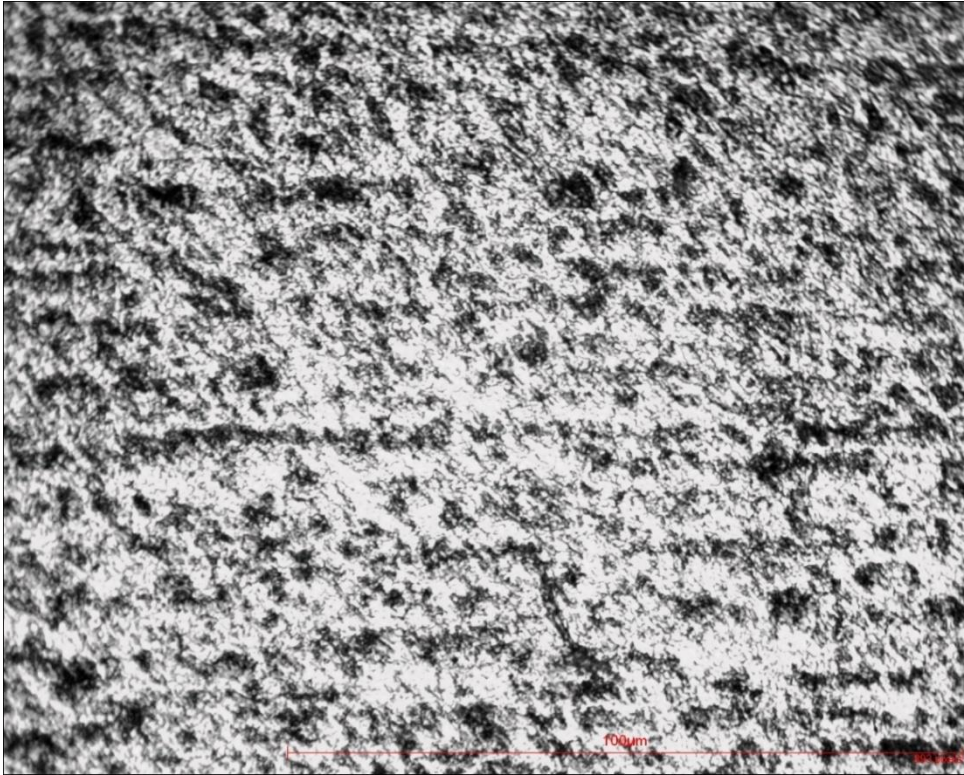
Figure 28. Base Metal Microstructure (400x)
