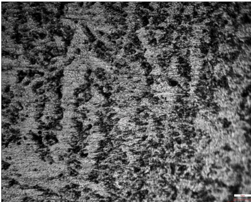
Figure 35. 390A Weld Zone Microstructure
