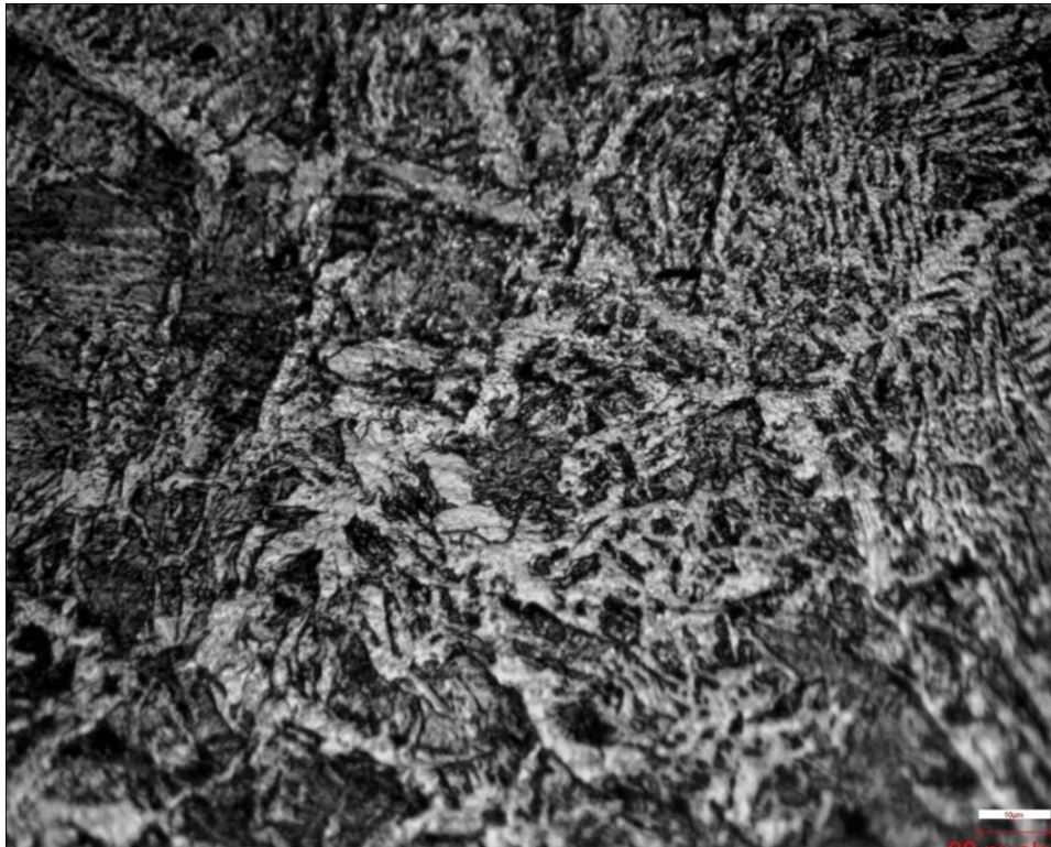
Figure 34. 350A HAZ Microstructure
