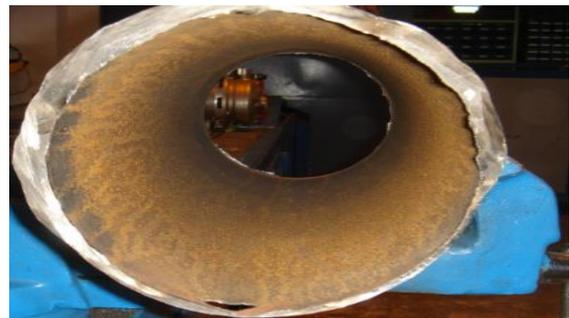
Figure 2-15 : Corrosion- Érosion, [46]
