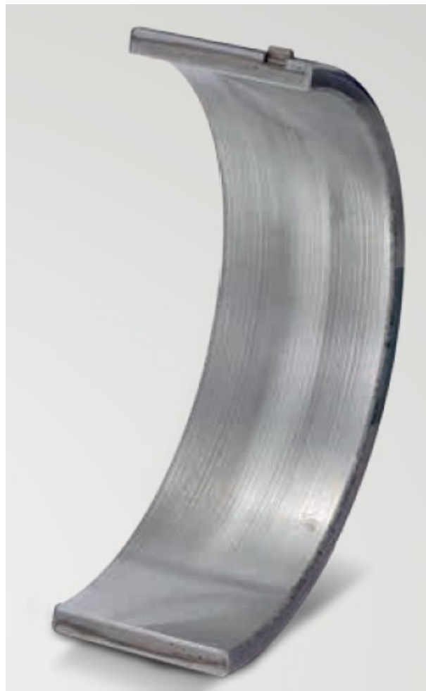
Figure I.21: Usure de rodage d'adaptation [42]
