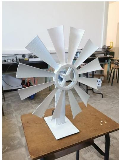
**Figure 4.2** Final Assembly of the windmill.
