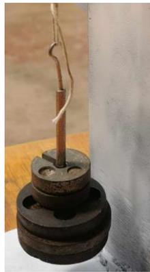
The weight plate is used to support the mass needed to be hung to neutralize the rotor moment.
