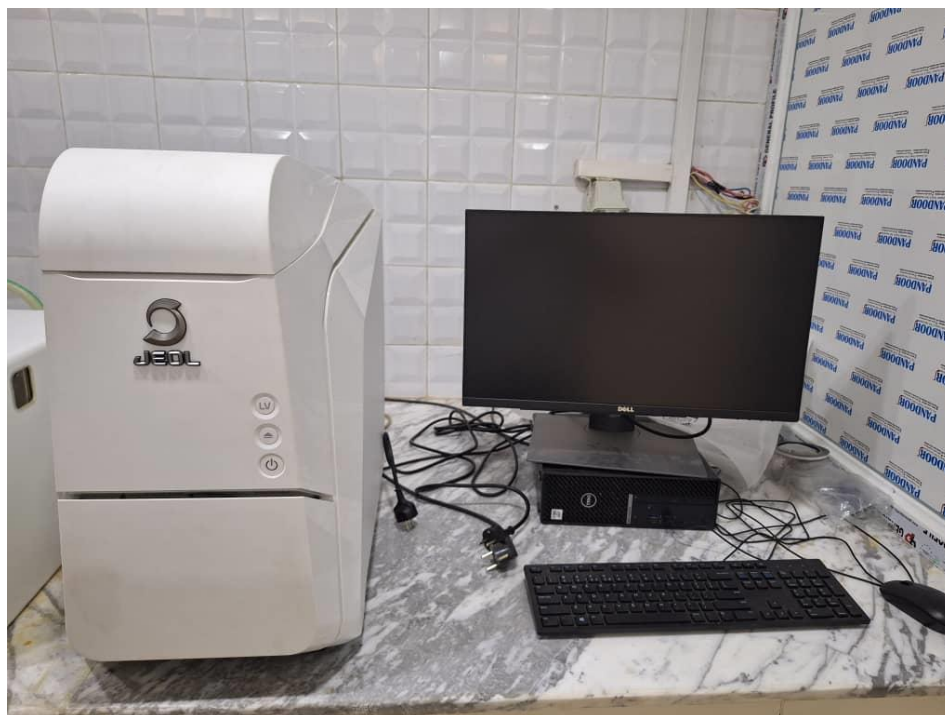
Figure 19: Scanning Electron Microscopy (Jeol-JCM-7000) (Mining engineering department).
