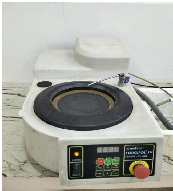
Figure 13:Polisher (materials engineering department)
