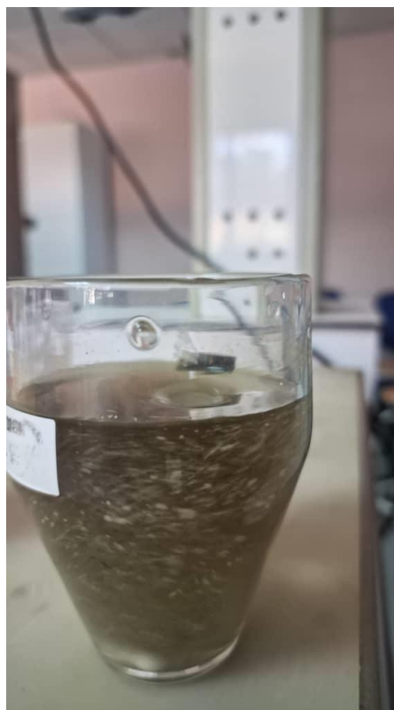
Figure 17: PANI/GO electrolyte before electrodeposition
