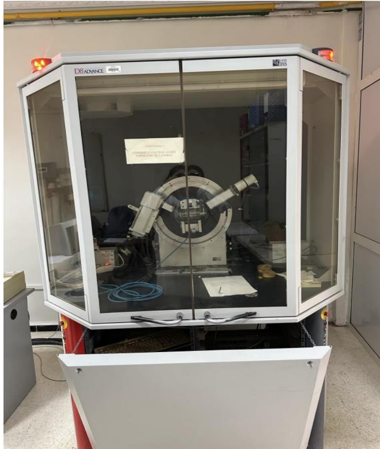
Figure 20: The XRD analysis (CDTA).
