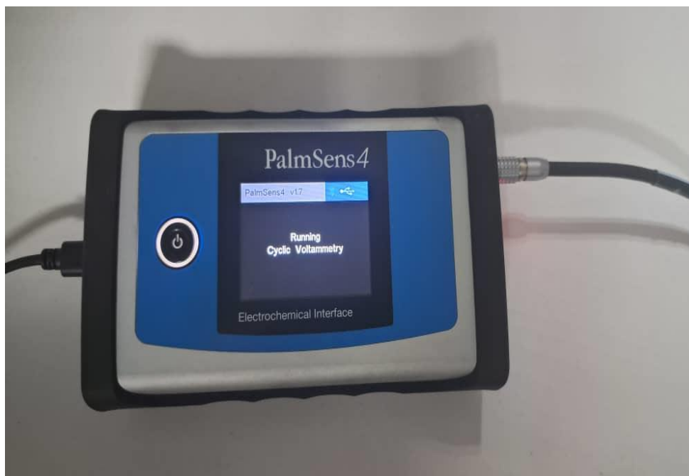
Figure 11: Potentiostat/ Galvanostat/ Impedance Analyzer
