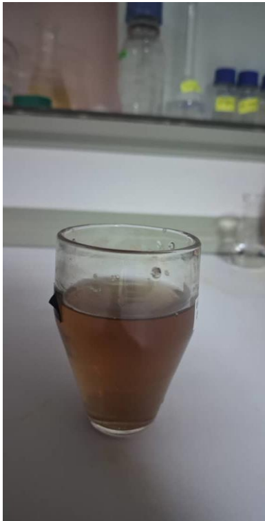
Figure 15: PANI electrolyte after stirring
