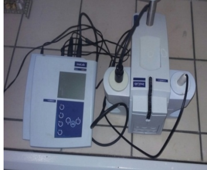
Photo 7: Multi-paramètres type WTW InoLab pH Level 1.
