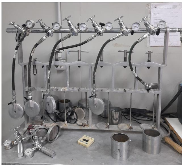
FIGURE 5.8 – Filter Press API model FANN
