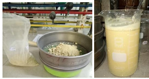
Figure 48:Tamisage(3.15mm). Figure 49:Pulpe.
