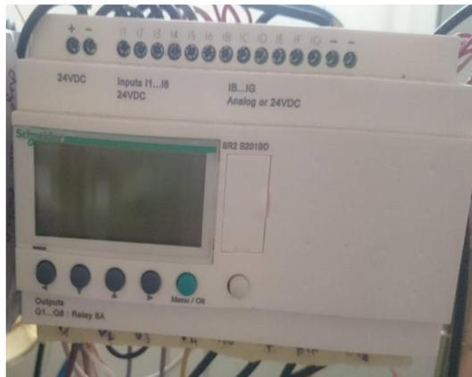
Figure 40 Automate programmable ZELIO (SR2 B201BD)
