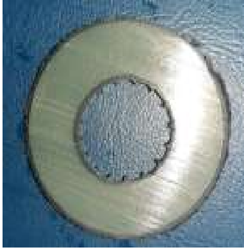
Fig 2: Cutting of cable insulation.
