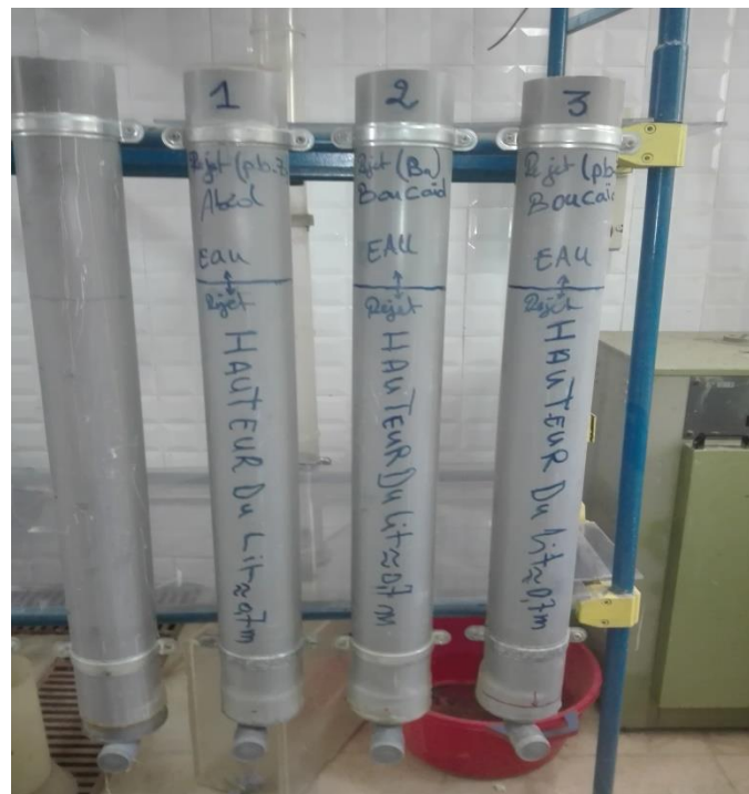
Figure IV. 9 – colonnes de lixiviation
