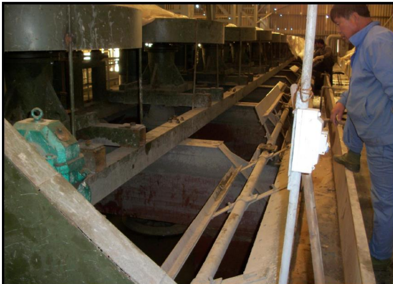
Figure III. 3 – Cellules de flottation.
