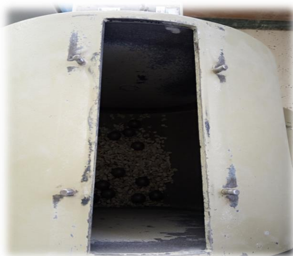
Figure 4-9 : La machine Los Angeles
