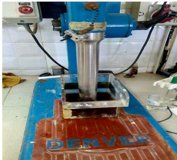
Figure 28 Cellule de flottation (Denver)
