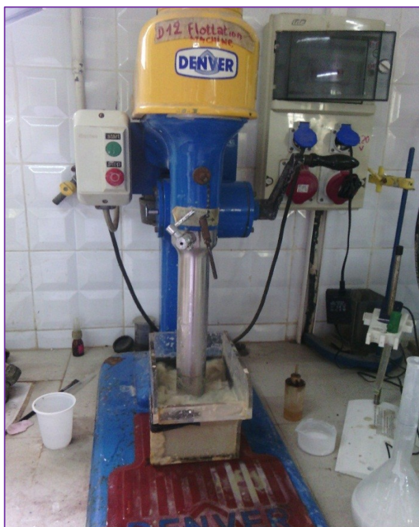
Figure 4-12 Cellule de flottation DENVER.
