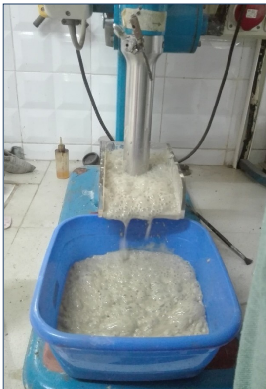
Figure 4-13 Essai de flottation de la bentonite.
