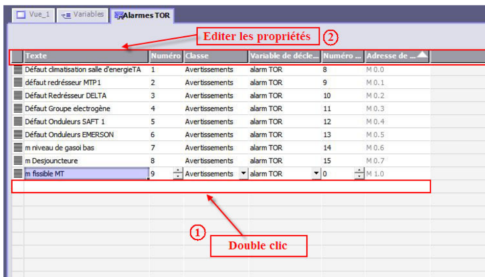
Figure III. 8. Configuration des alarmes TOR (2).
