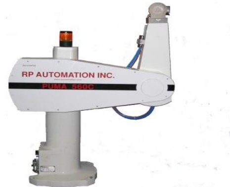
FIGURE 1.2: Robot de type PUMA.
