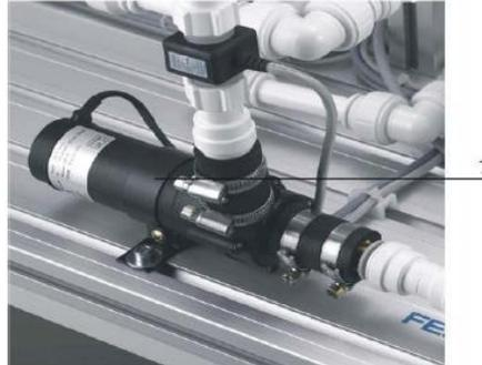
*Figure I.4: Pompe centrifuge.*
