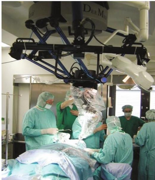
Figure 1.14 Le SurgiScope, un robot Delta portant un microscope de 70 Kg (Isis France) [Bri]
