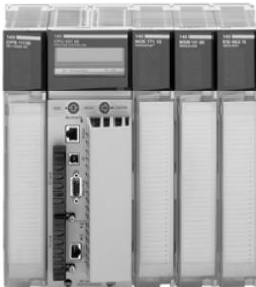
Figure A.7: Automate Modicon Quantum
