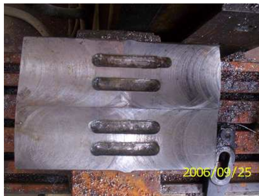
Figure III.4 : Rainurage du rail.
