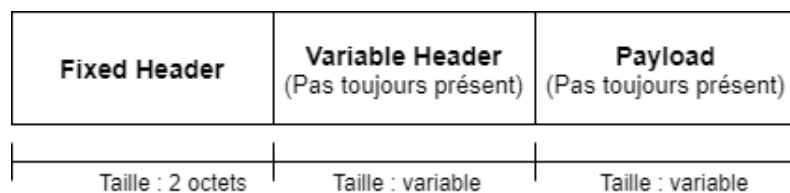
FIGURE 4.3: Format des paquets MQTT
