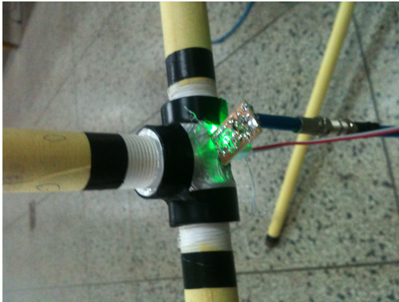
Figure 3.11: LNA module outside the shielded casing
