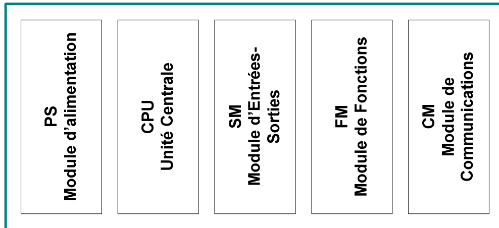
Figure I.A.1 Architecture d'un Automate Programmable
